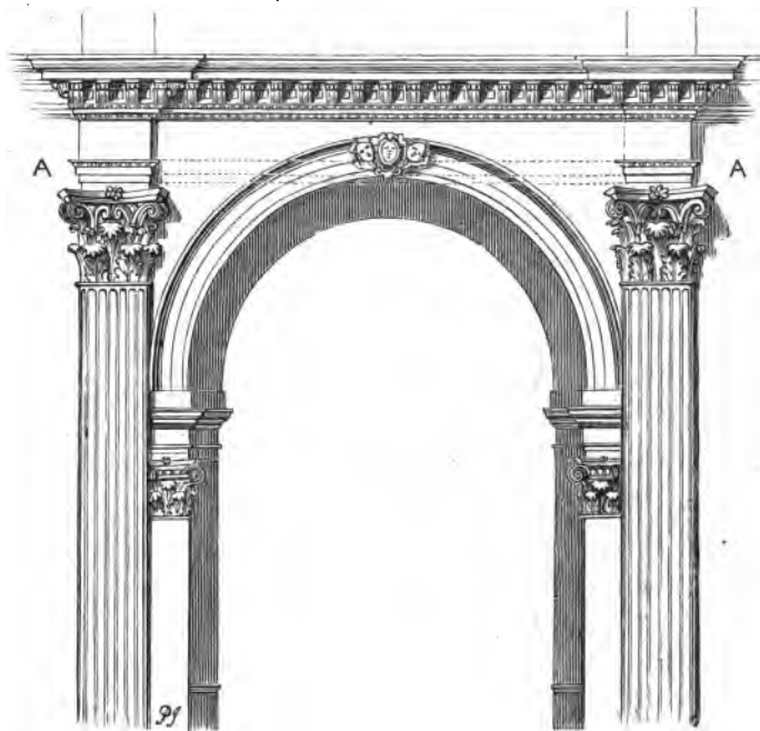
PIER ARCHES OF THE NAVE, SHOWING THE ARCHIVOLTS, RISING ABOVE THE ARCHITRAVES.
